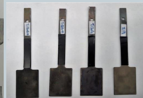
Ti anodes with catalyzing coatings
